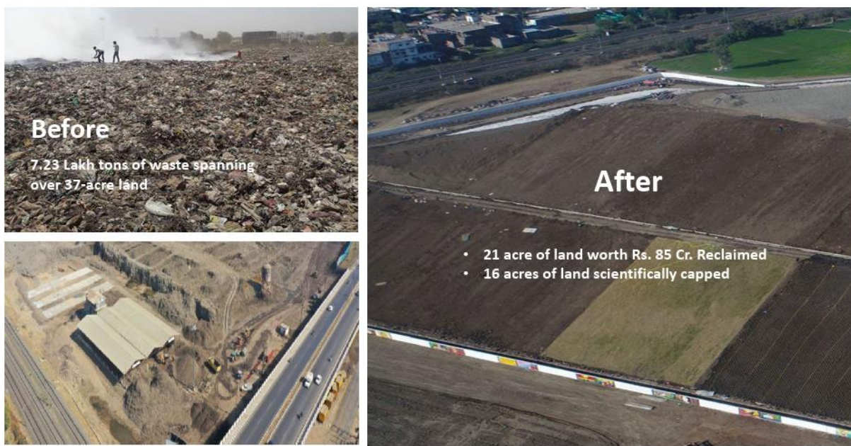
Figure 20 Transformation of Bhanpur Khanti Dumpsite
